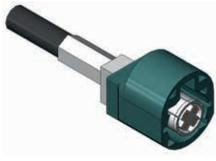
The F819 combines several advantages: Conical inlet of the external as well as internal contact for better contacting and compensation of tolerances. In addition, the screwed internal contacts (F17512B0023G150SPS1) prevent the contact from being pulled out of the receptacle. The probe is used for purely electrical contacting of HSD females.
